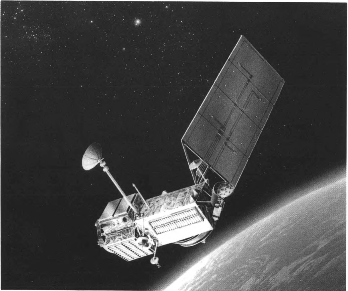
This is an artist's conception of the US/ French TOPEX/ Poseidon satellite designed for precision (to an accuracy of several centimetres) measurements of ocean surface topography during the period 1992 to 1995, and possibly longer. (Courtesy of NASA.)
