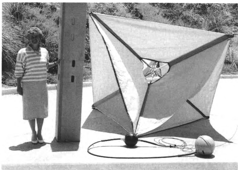
These surface drifters were developed for WOCE and TOGA. (Courtesy of Peter Niiler.) Each Tristar Drogue is compactly packaged in a cardboard box to be assembled on board the ship before being released into the ocean.
