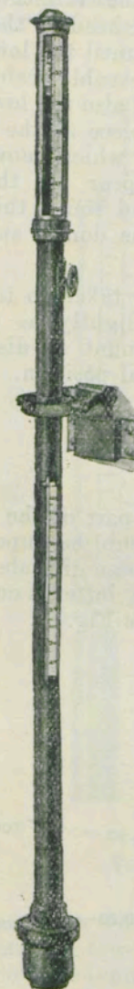
FIG. 3.—KEW PATTERN BAROMETER.
