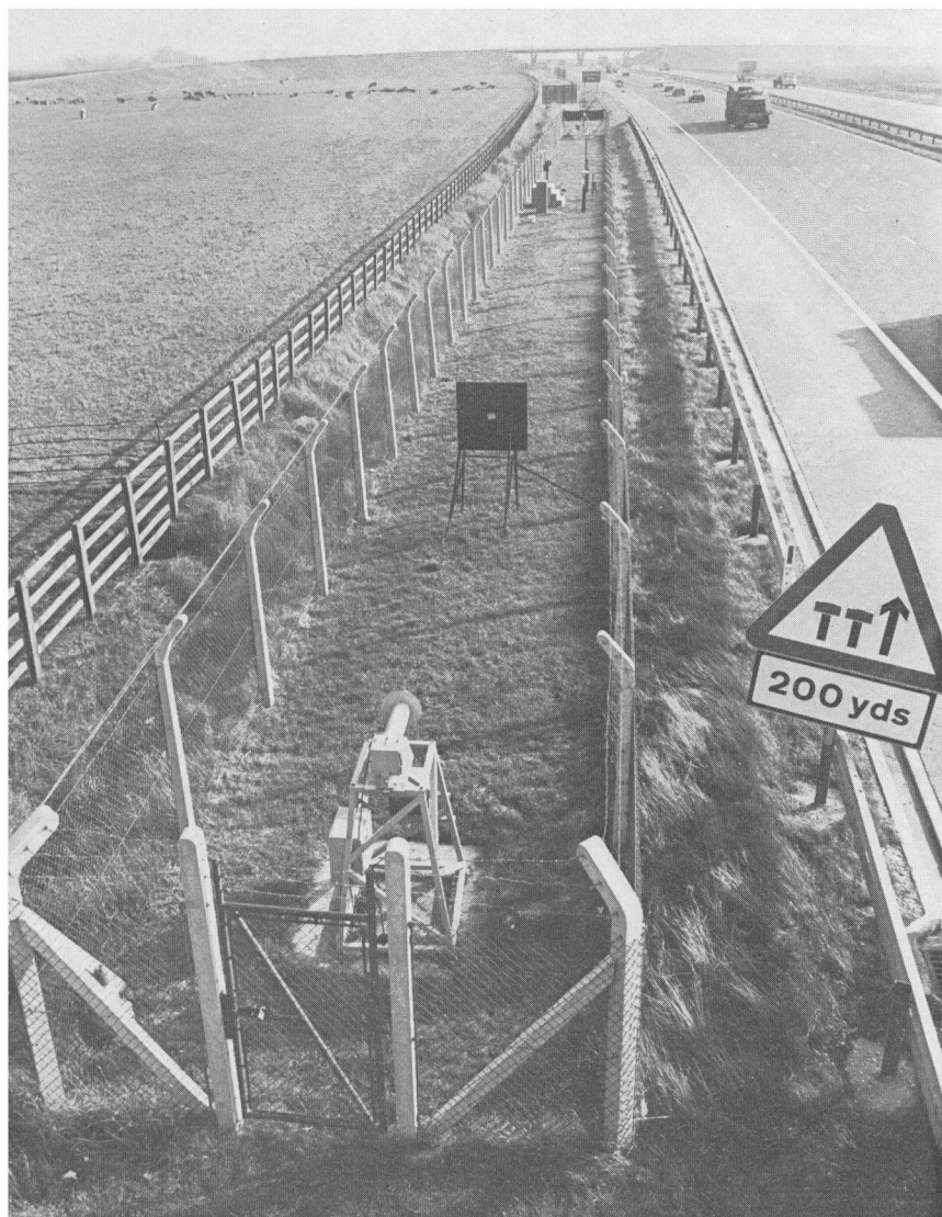
PLATE II—THE METEOROLOGICAL OFFICE TRANSMISSOMETER
