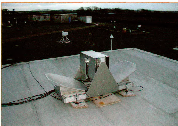
Figure 5. Deployment of the cloud radar at Camborne, with the microwave radiometer visible in the background.
