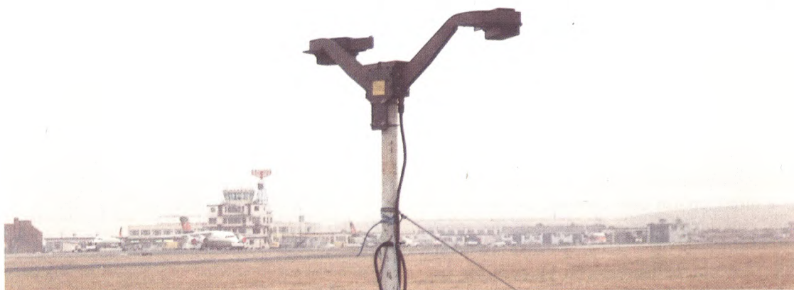
Figure 2. The HSS forward scatter visibility meter.
