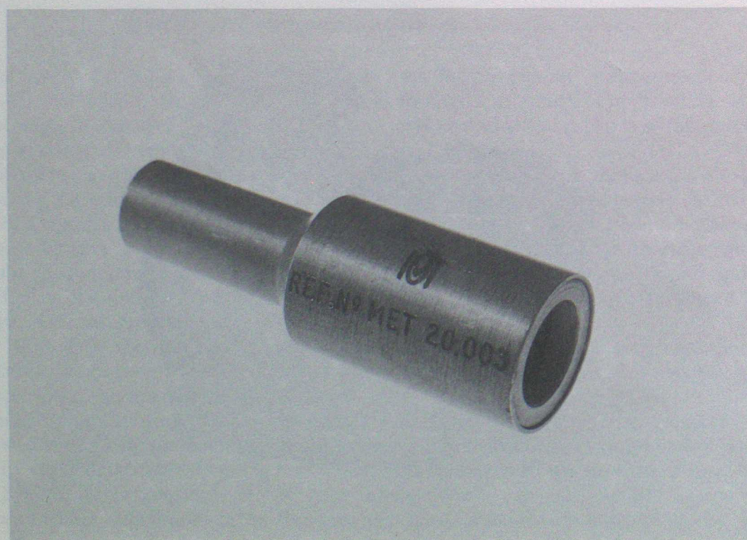
Plate IV. Damping cap for precision aneroid barometer. Illustrated at approximately twice full size.
