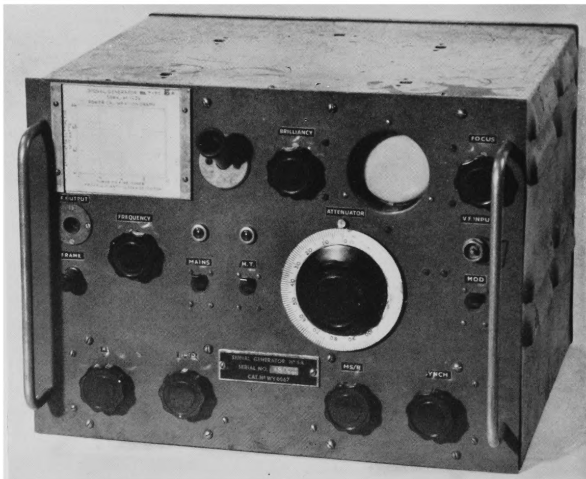
SIGNAL GENERATOR NO. 6A, FOR MEASURING RECEIVER PERFORMANCE OF METEOROLOGICAL OFFICE RADAR, TYPE 1
