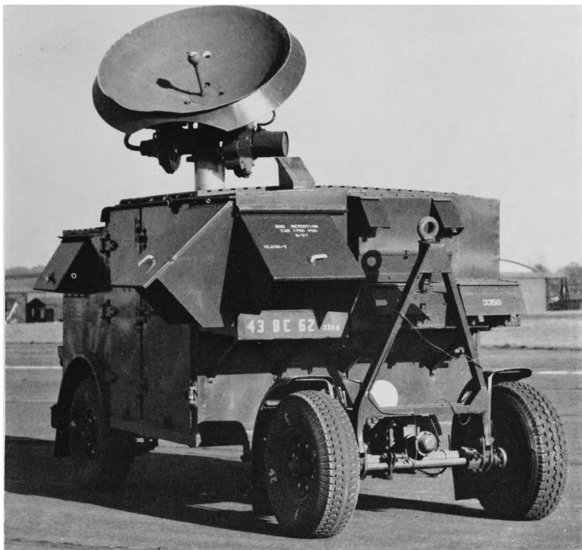
GENERAL VIEW OF METEOROLOGICAL OFFICE RADAR TYPE 3 (MODIFIED A.A. NO. 3 MARK 7)
