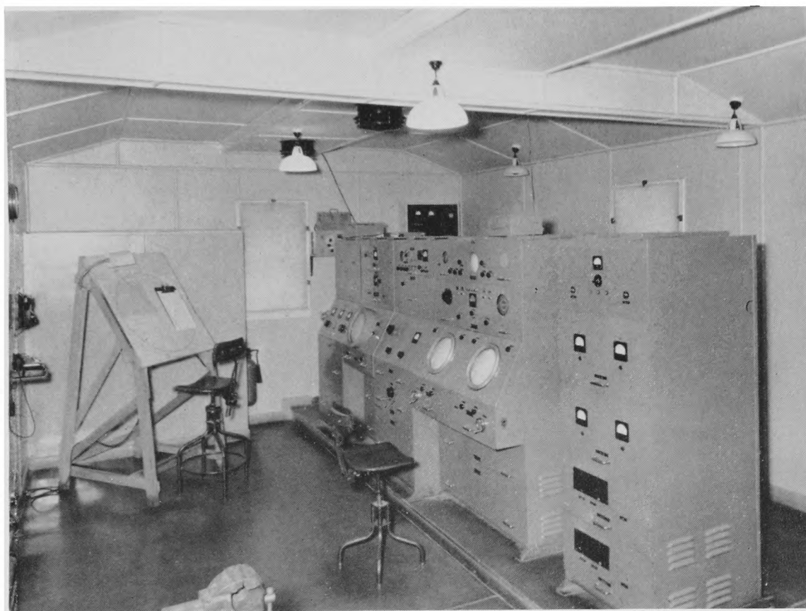
NEW ZEALAND WIND-FINDING RADAR, TYPE M.E.7
