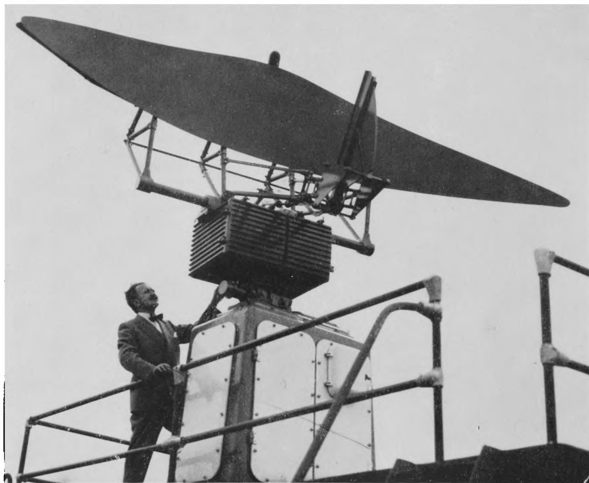
SCANNER UNIT OF DECCA STORM WARNING RADAR, TYPE 41
