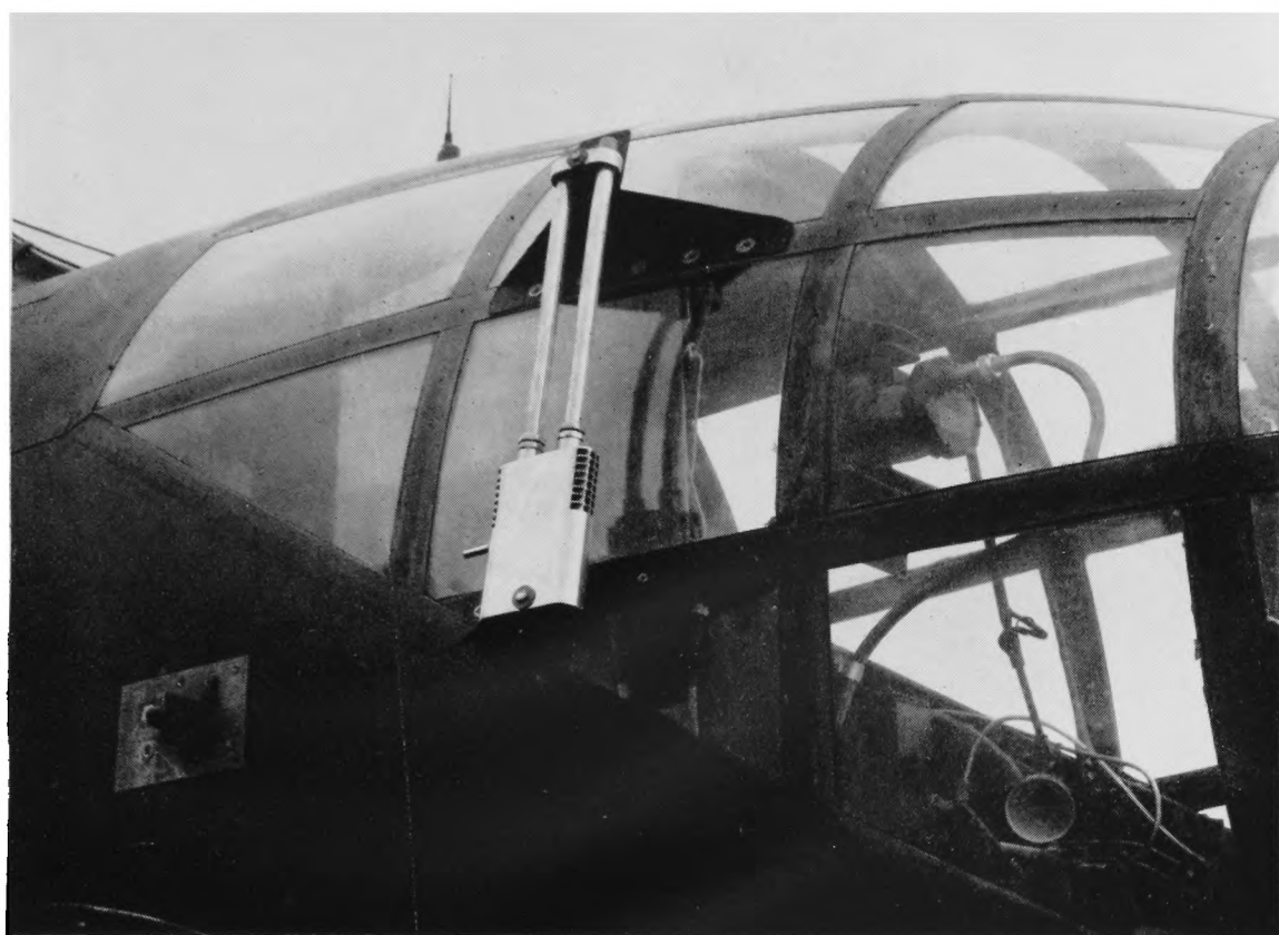
INSTALLATION OF PSYCHROMETER, MARK 6, ON A BOSTON AIRCRAFT
