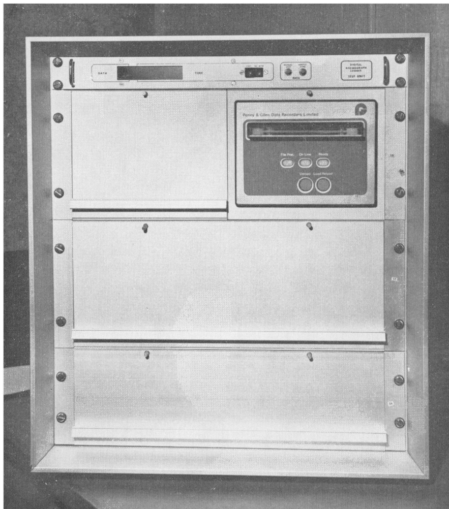
PLATE I—DIGITAL ANEMOGRAPH LOGGING EQUIPMENT (DALE)
