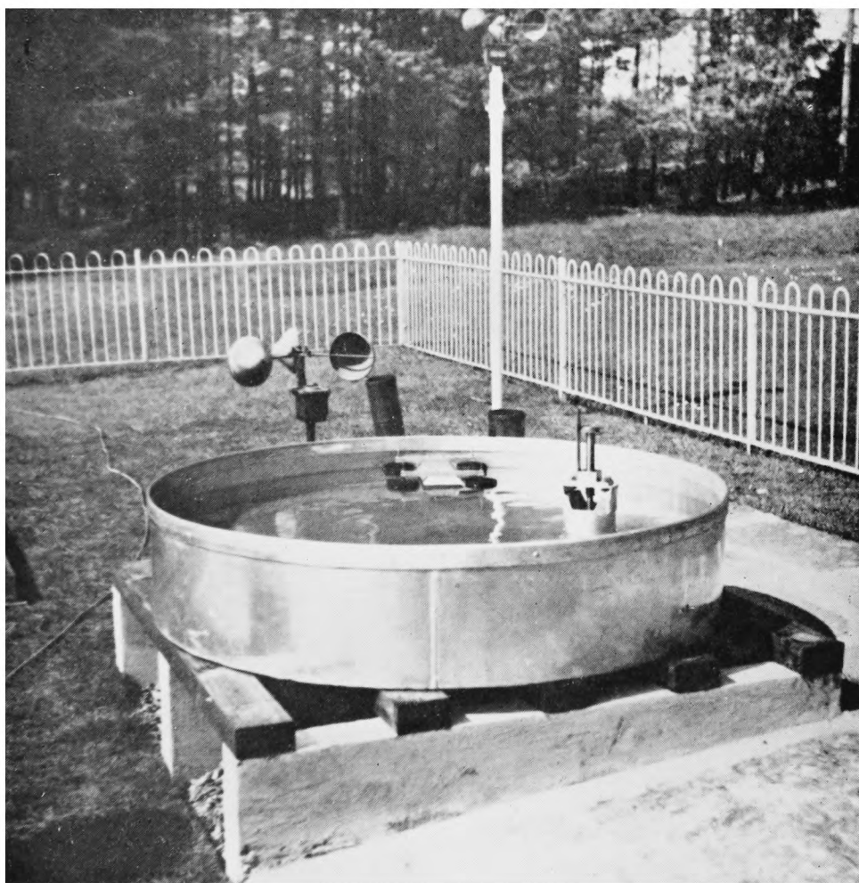
EVAPORATION PAN AT STOCKS RESERVOIR United States Weather Bureau class A type.
