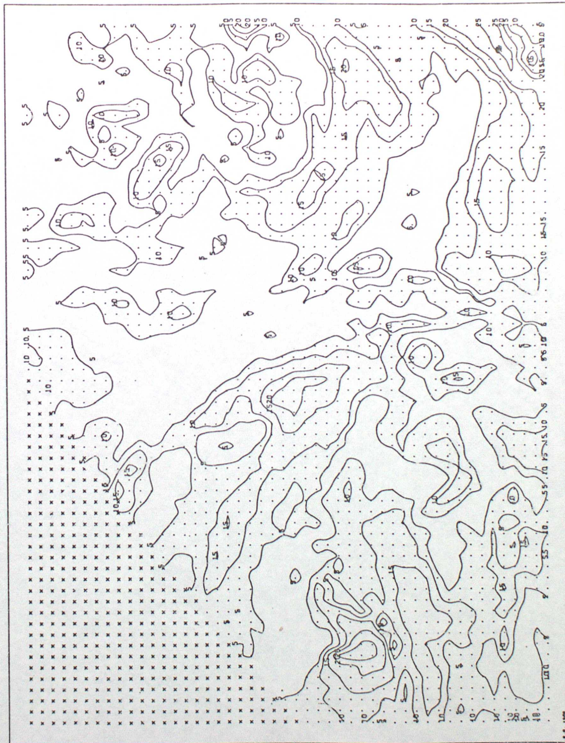
Figure 4 Absolute difference between measured radiances and radiances calculated with initial humidity field
