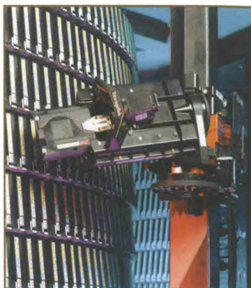
Inside the MASS tape library, a grabber is transferring one of over 2,500 state-of-the-art cartridges
