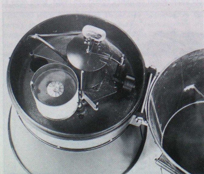
Tilting-siphon rain recorder
