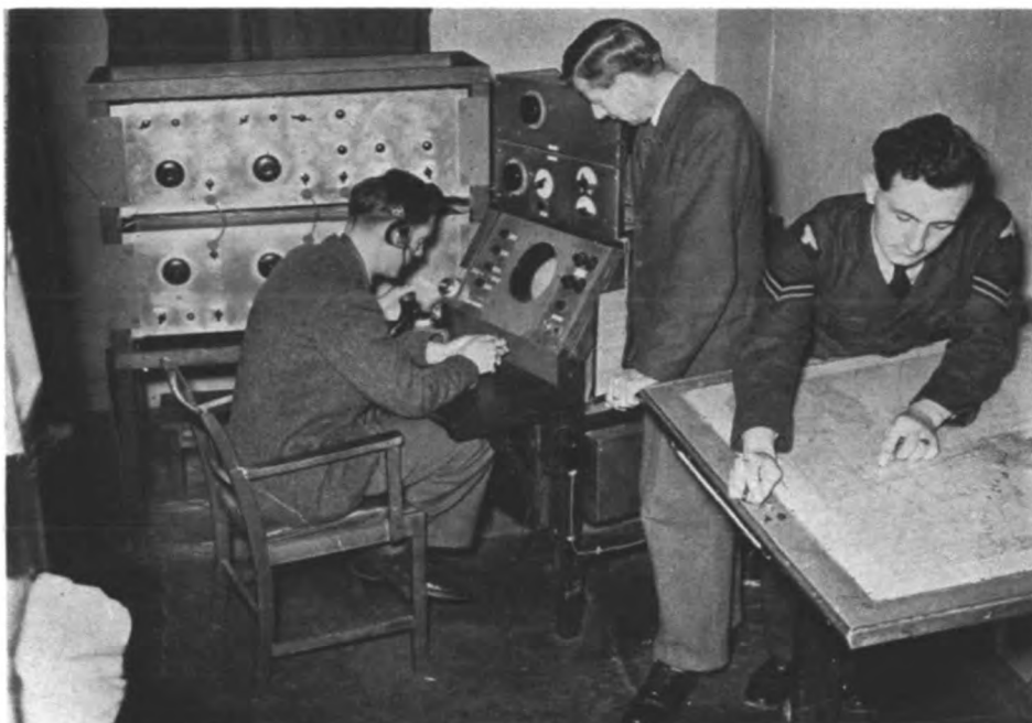
Fig. 1—Sferic set showing amplifiers, cathode-ray tube and plotting table
