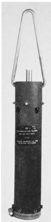
FIG. 9 The rubber sea-temperature bucket
