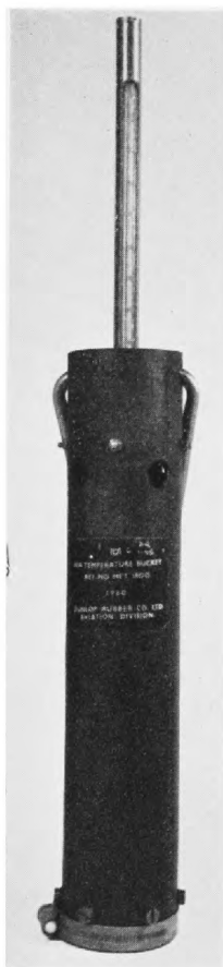
FIG. 9 The rubber sea-temperature bucket
