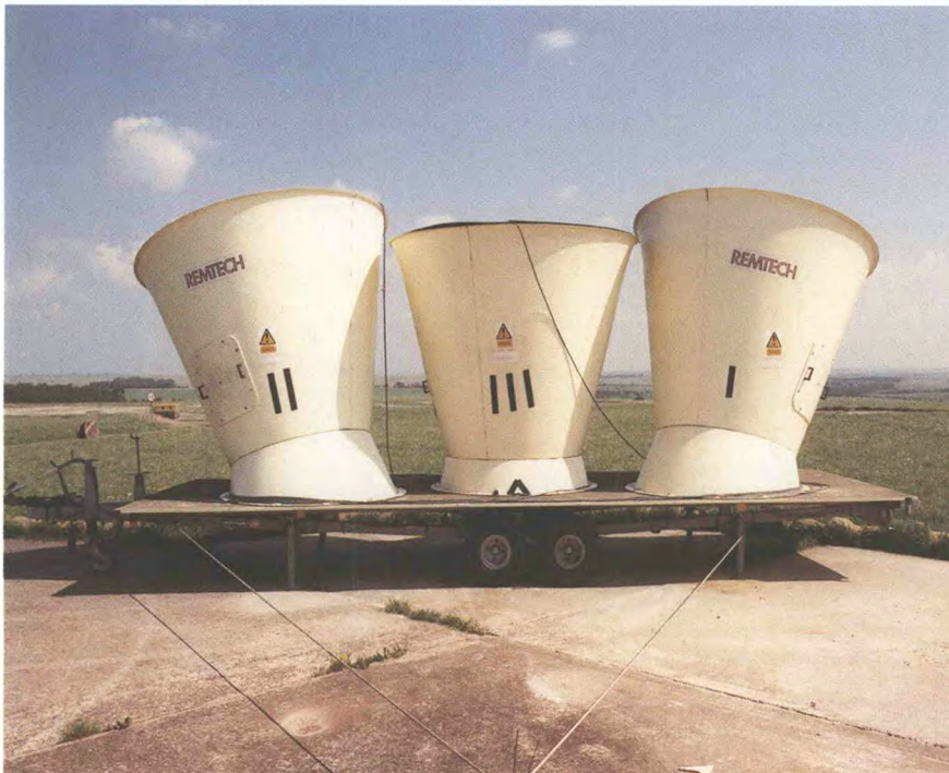
Doppler acoustic sounder used in the wind-finding trial at Larkhill
