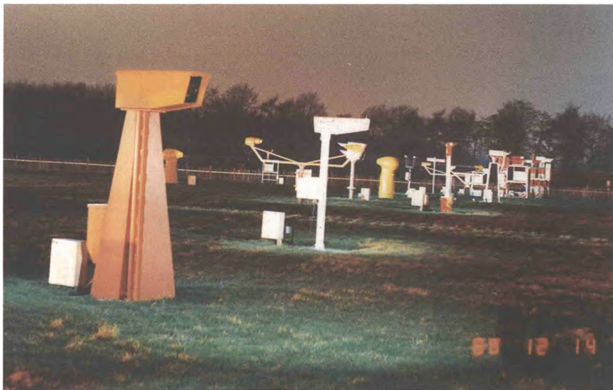
Instruments used in the international intercomparison of visibility measurements at RAF Finningley
