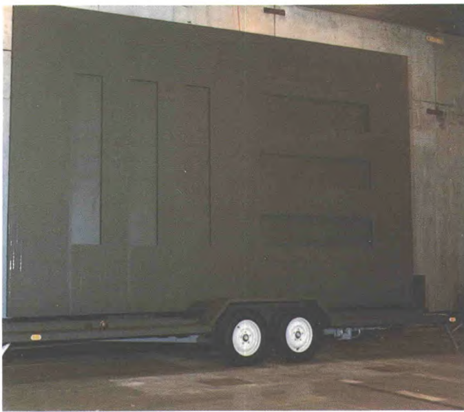
The instrumented target at Boscombe Down which simulates the thermal signature of a battle tank
