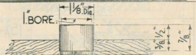
FIG. 6. METHOD OF FITTING AIR VENTS.
