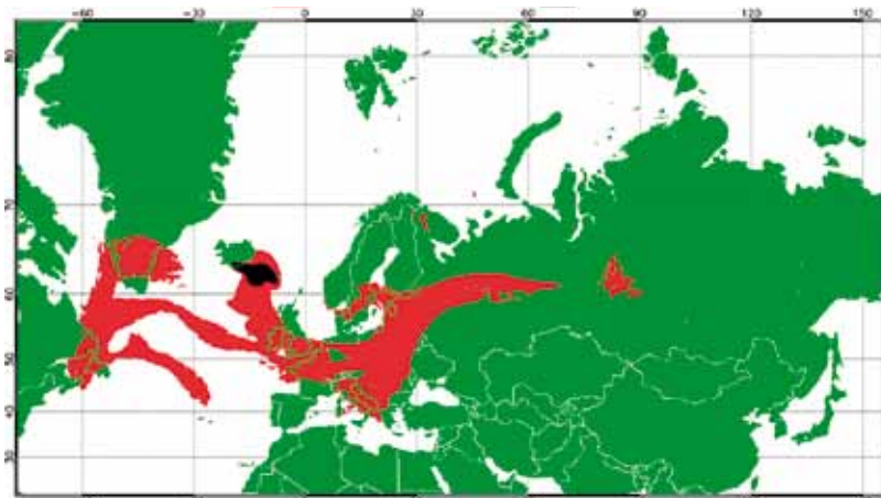
Volcanic ash chart – the red zones represent the standard safety threshold, while the black represents ash concentrations that are 20 times higher than the standard (red) threshold. The black zone is the area within which aircraft engine manufacturer tolerances are exceeded.
