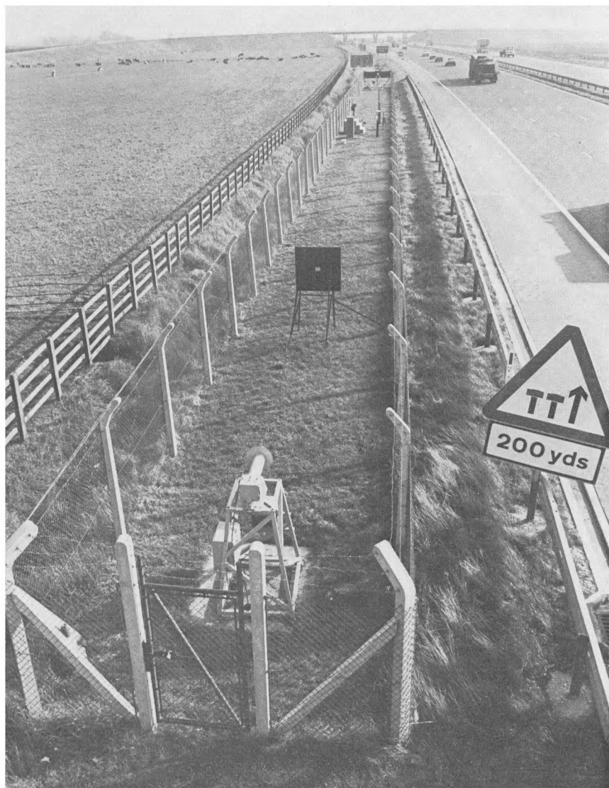
PLATE II—THE METEOROLOGICAL OFFICE TRANSMISSOMETER
