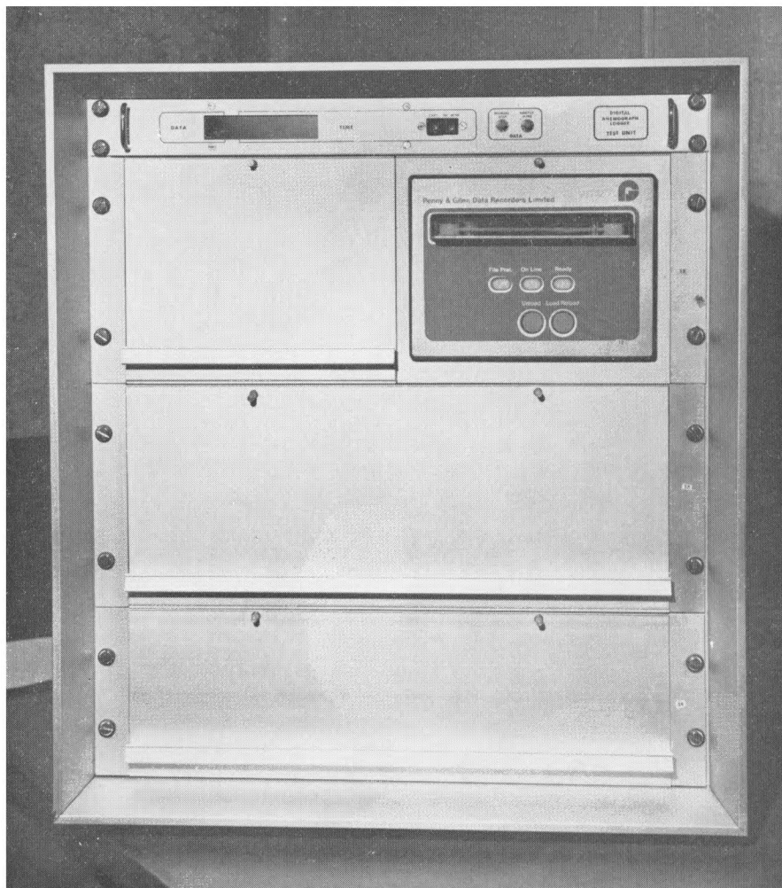
PLATE I—DIGITAL ANEMOGRAPH LOGGING EQUIPMENT (DALE)
