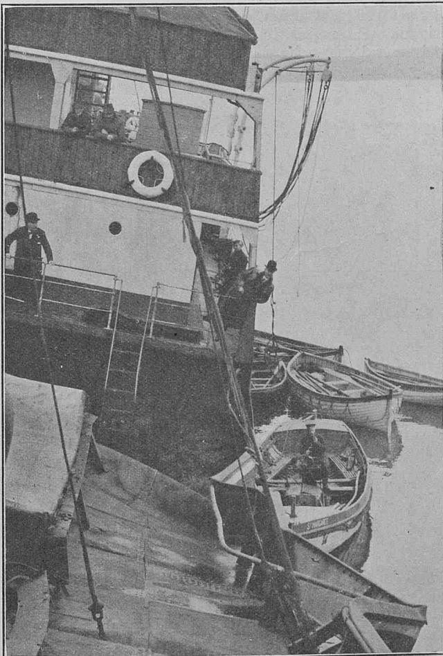
The buckled fore deck, hatch coamings and bulwarks of the Porthcawl .
