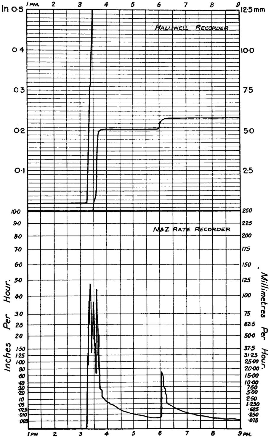
The distortion of the trace thus produced is a characteristic of the instrument, and one cannot be sure to what extent this process goes on whilst rain is falling as well as after its cessation. Any checking by comparison with an ordinary gauge is also effectively prevented by this distortion.
