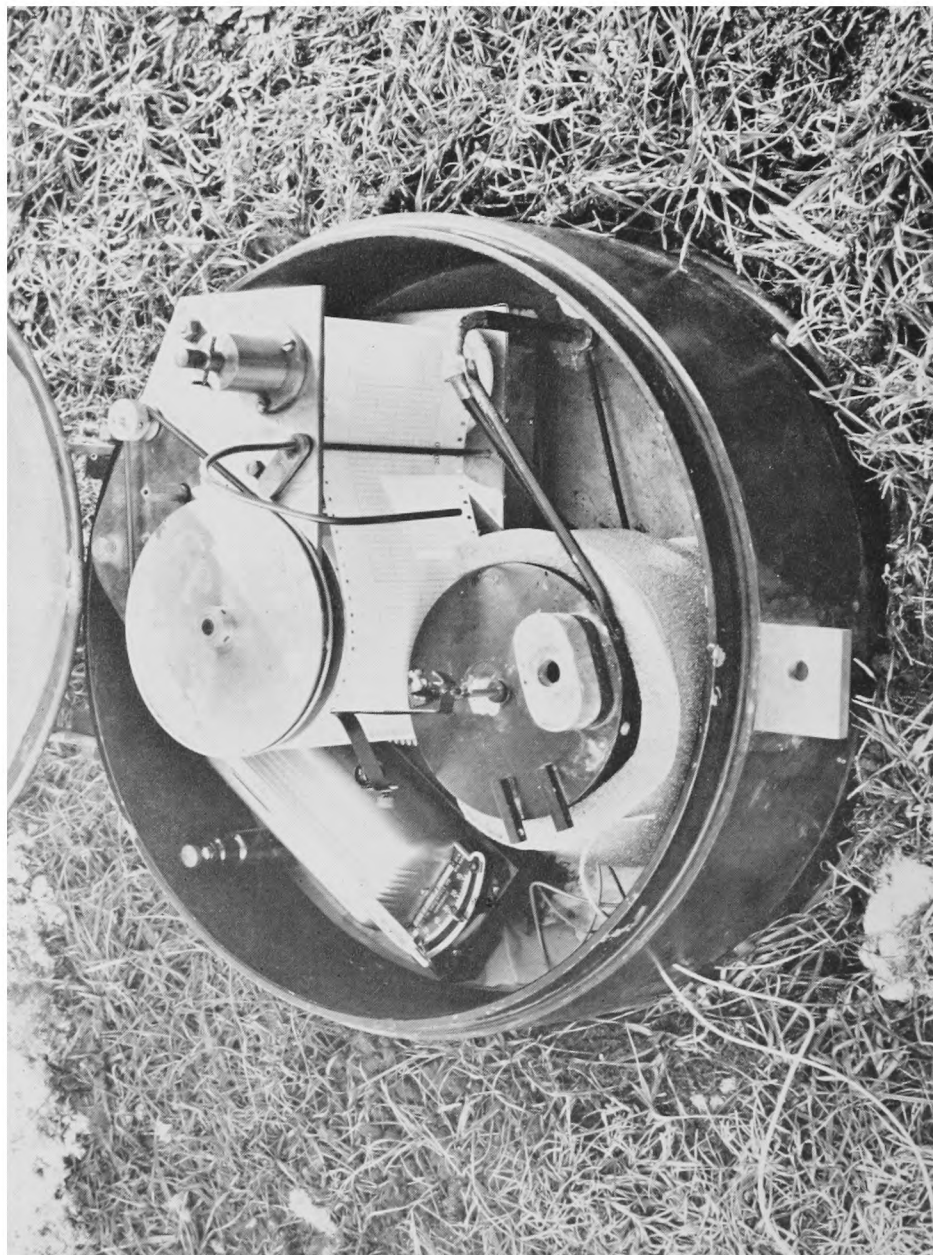
PLATE II—MODIFIED RAIN-RECORDER WITH EIGHT-DAY STRIP CHART MECHANISM, EQUIPPED WITH LOW-VOLTAGE HEATING AND WALL THERMOSTAT Note the lagging round the chamber. (See p. 337.)
