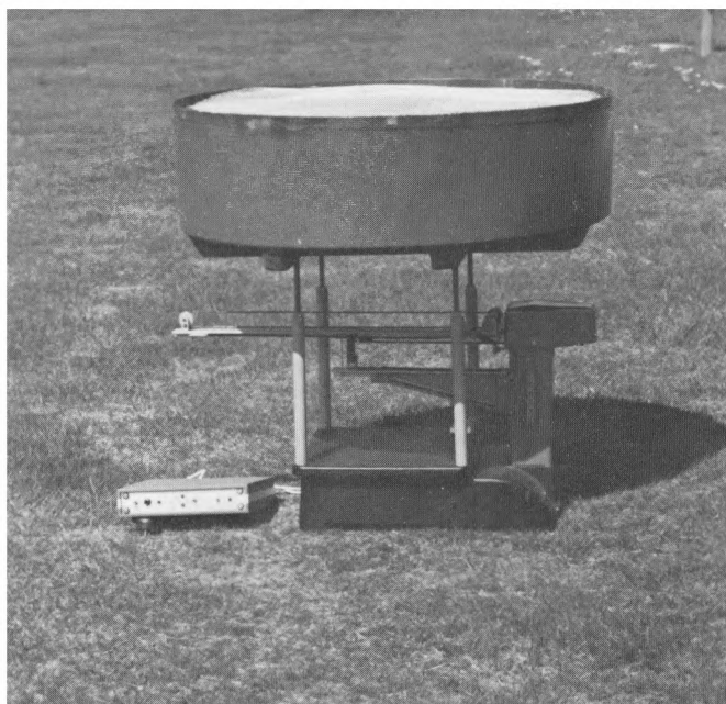
Plate I. The gravimetric rain-gauge complete with control electronics. The top pan is 90 cm in diameter. (See facing page.)
