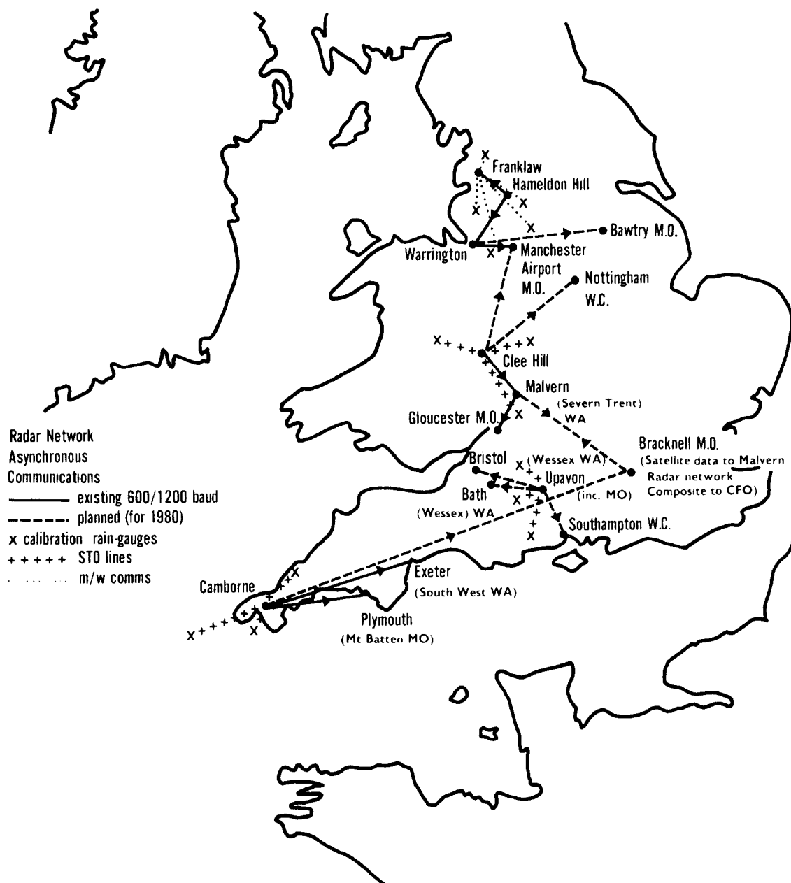
Figure 2. Illustration of the communication-line network connecting various existing (solid line) and planned (dashed line) users to the radars. All the lines shown carry 3-bit data and are land-lines leased from the Post Office and operated at a data rate of 600/1200 baud.
