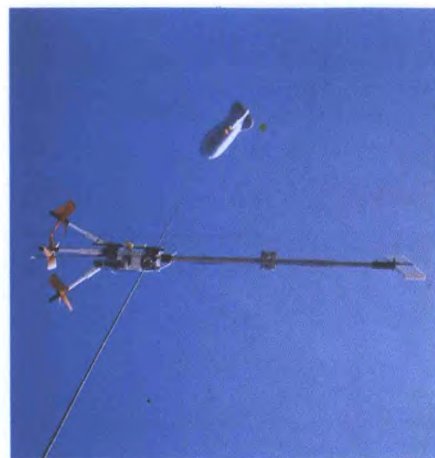
Turbulence probe mounted on the tethering cable of a kite balloon.
