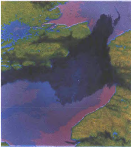
Composite night-time image of south-east England derived from two spectral channels. The grey-shaded areas indicate fog or low cloud and other colours show temperature variations. The London 'heat island' and the variations in sea surface temperatures are clearly apparent.
