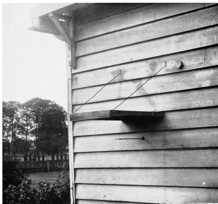
FIG. 5 — EXPOSURE OF COLLECTOR OF HIGH-RANGE POTENTIAL GRADIENT RECORDER.
