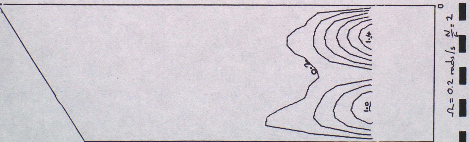
Figure 5.13 Cross-sections of the annulus gap showing the vertical penetration of the topographically forced wave at different rotation rates. On the base there is a wave 3 topography with radial variation and an amplitude 15% of the depth.
