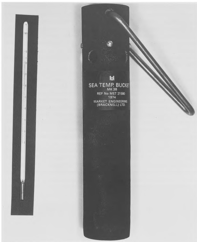
Figure 15. Sea temperature bucket and thermometer.
