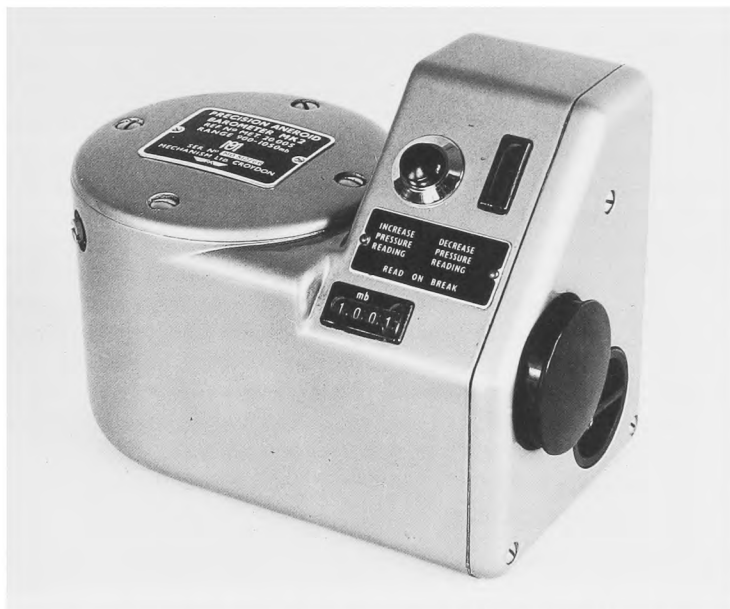
Figure 1. Precision Aneroid Barometer Mk. 2 — general view. Note the housed static vent on left side beneath cap.
