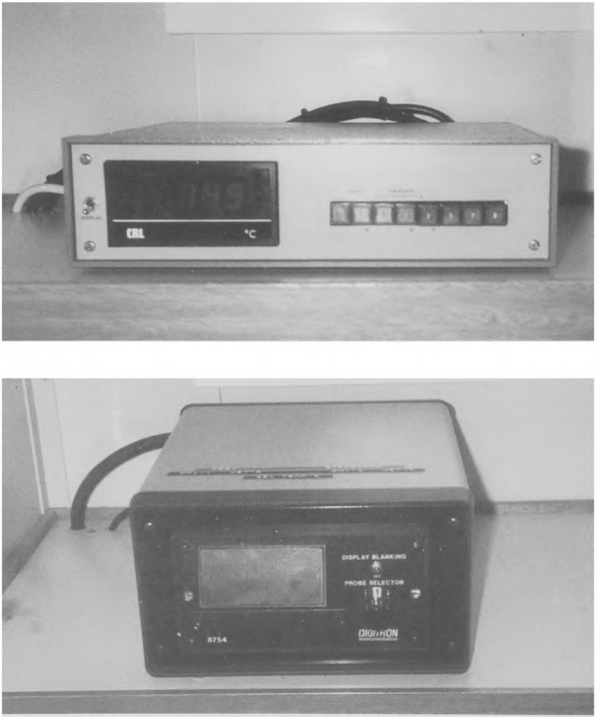
Figure 13. Digital Temperature Indicators. Top Mk. 1B. bottom Mk. 2.
