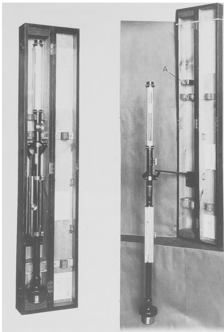
Figure 6. The Kew-pattern marine barometer and its stowage.
